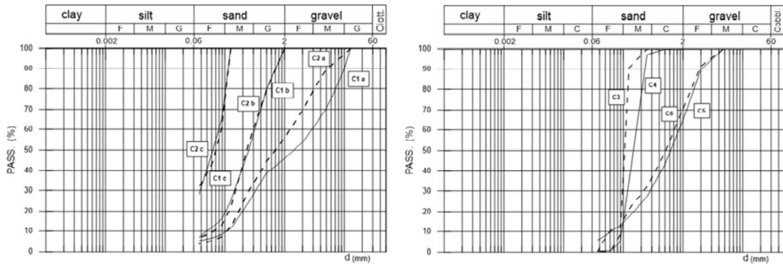
Fig.2. Size distribution of samples tested in laboratory.
