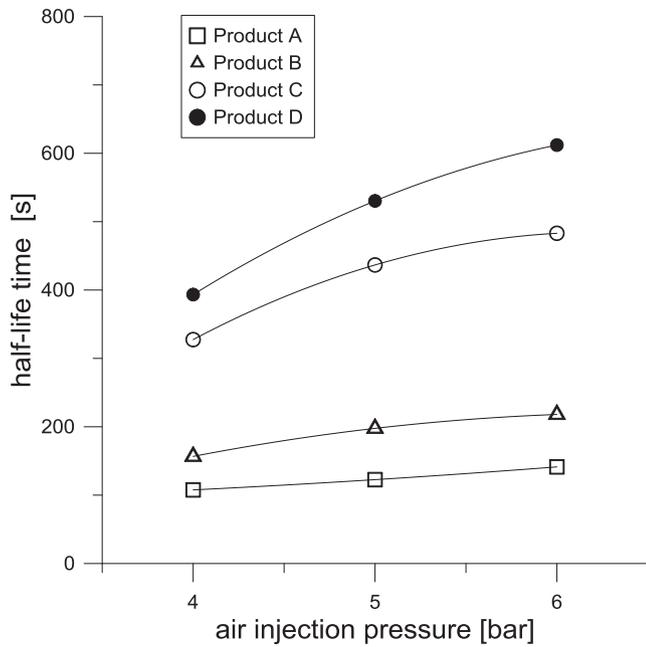
Fig. 4. Average values of  $hlt$  for  $Cf = 2.5\%$  and  $FER = 12$ , as a function of injection pressure.
