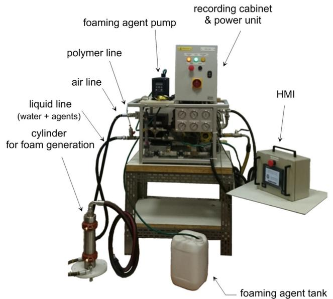
Fig. 2. Main components of the laboratory foam generation system.
