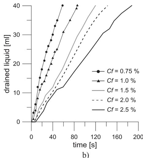
Fig. 5. Typical results of half-life tests: (a) effect of  $FER$  for a foam generated using Product B with  $Cf = 2.5\%$  and (b) effect of  $Cf$  for a foam generated using Product C with  $FER = 12$ .
