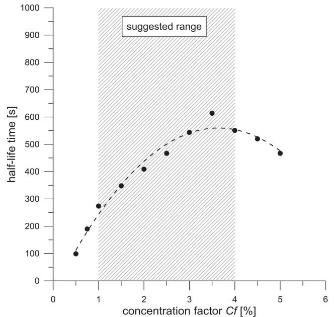
Fig. 6. Typical evolution of the half-life time with  $Cf$  measured for Product C.
