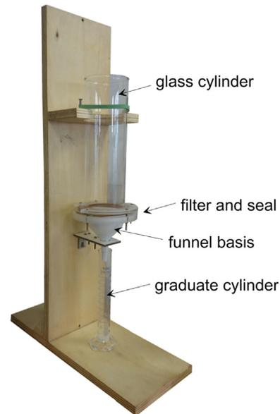
Fig. 3. Half-life test laboratory apparatus.
