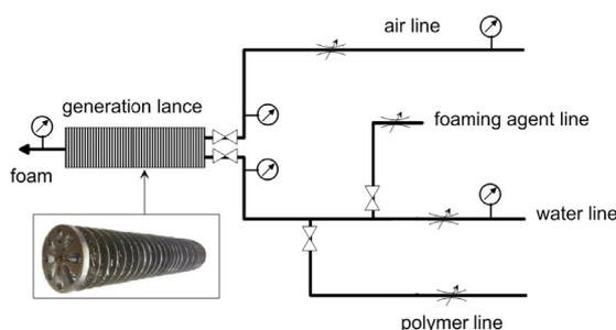
Fig. 1. Laboratory foam generation system.
