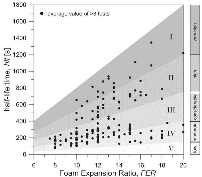
Fig. 10. Foaming product classification based on the stability of the generated foam.
