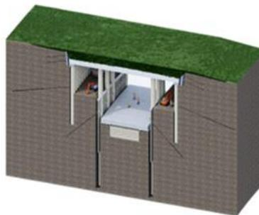
5) Execution of the main axis slab and covering of the tunnel
