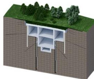
6) Completion of the structure and demolition of intermediate piles
