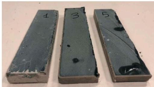
Figure 4. Pictures of sections of samples sawn after exposure to air at different values of relative humidity, from the left: 50%, 90% and 98%.
