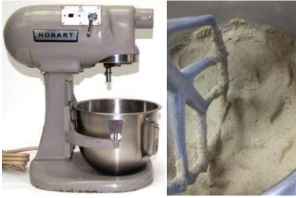
Figure 5 Hobart mixing apparatus and mixing tool (modified after Sebastiani et al., 2017).
