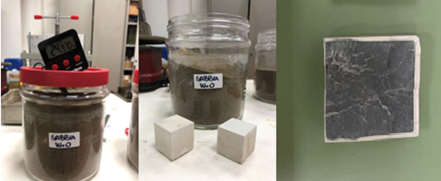
Figure 4. Curing in soil. Aspect of the internal surface of a sample showing external discoloring
